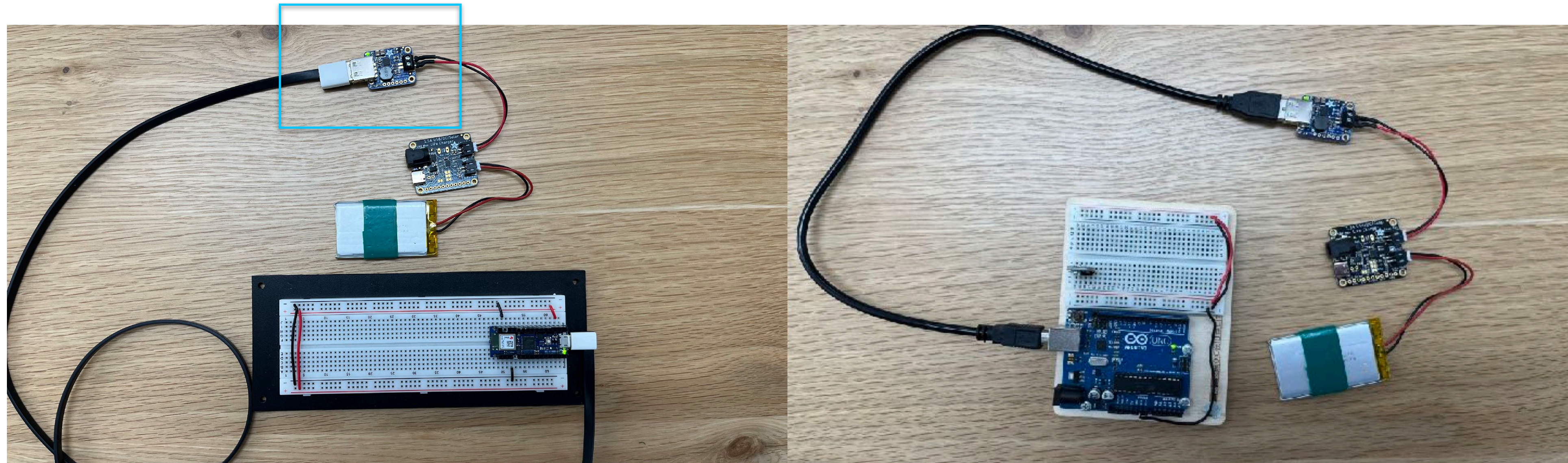
With PowerBoost 1000, 1.8-4V to 5V@1000mA output
